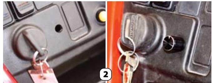
2) We located an area on the dash to mount our volume control knob and drilled a hole, mounted the controller, and connected these two together and pulled the loose wires under the hood to the front of the vehicle that we will later connect to our amp.
