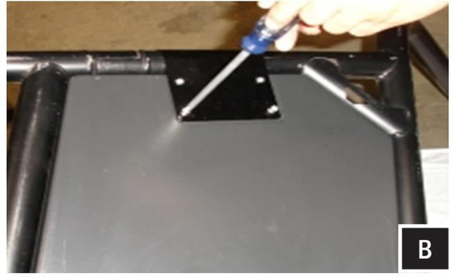
B. While holding the enclosure securely in place, loosely install the 2 brackets using the screws provided.
