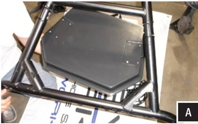
A. With one person on either side of the vehicle place the WP3-RZOA into location from the underside of the cage
