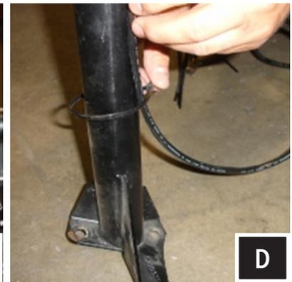
D. Using the zip ties provided, route the Power/Ground loom to the battery location away from any moving parts or sharp metal. NOTE: The 4 pin short cable is for additional speakers (WP3-RZOA+2) and the 4 pin long cable is for adding an SSV Works Powered Subwoofer (Part# WP-RZS10)
