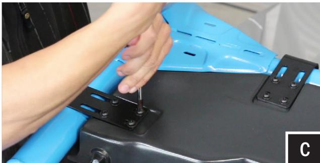
C. Once the enclosure is centered side to side, press the bracket toward the center of the vehicle and tighten the brackets using the #3 screwdriver.
