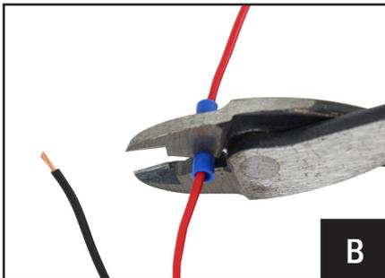
B. Crimp the supplied fuse holder onto the end of the RED wire and attach to the battery "+" terminal.
