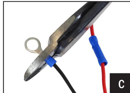
C. Crimp the supplied ring terminal to the BLACK wire and attach to the battery "-" terminal.
