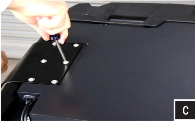
C. Once the enclosure is in position, press the bracket toward the center of the vehicle and tighten the brackets using the #3 screwdriver. NOTE: After all brackets are tightened, it may be necessary to go back and re-adjust the brackets to ensure the enclosure is properly secured.
