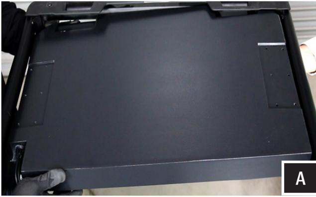
A. With one person on either side of the vehicle place the WP-RZ304 into location from the underside of the cage.
