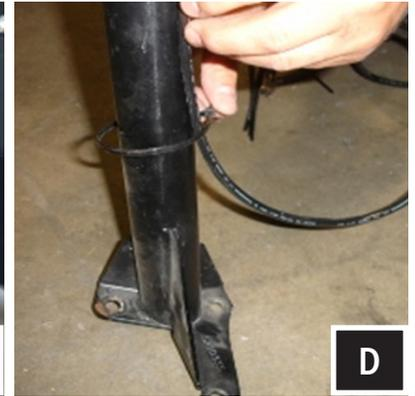
D. Using the zip ties provided, route the Power/Ground loom to the battery location away from any moving parts or sharp metal. NOTE: The 4 pin short cable is for additional speakers (WP-RZ30+2) and the 4 pin long cable is for adding an SSV Works Powered Subwoofer (Part# WP-RZ3GBS10 or WP-RZ3BSS10)
