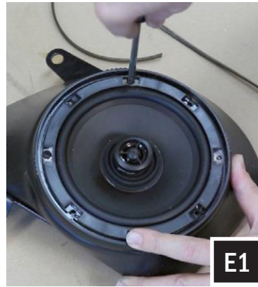
E. Connect the speaker harness to the enclosure harness and use a screwdriver secure the speaker to the pod (E1) Place the loaded enclosure in location for mounting (E2).
