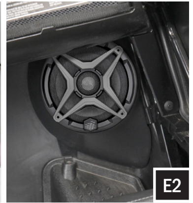
E. Connect the speaker harness to the enclosure harness and use a screwdriver secure the speaker to the pod (E1) Place the loaded enclosure in location for mounting (E2).
