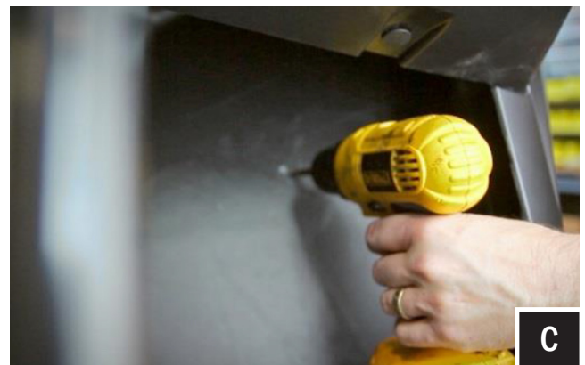
C. With a 1/4" drill bit, drill the screw hole for mounting the speaker pod.
