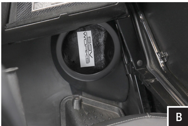
B. Set the unloaded pod in place and mark the top mounting location with a scribe or punch tool on to the floorboard.
