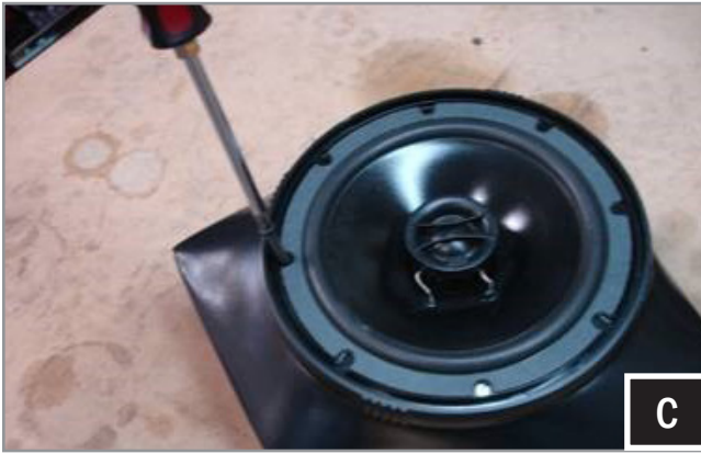
C. Connect and install the speaker into the enclosure (be sure to connect the “+” red speaker wire to the “+” terminal on the speaker and the “-“ black speaker wire to the “-“ terminal on the speaker) using the #2 Phillips screwdriver.
